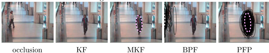
c) In the sequence "EnterExitCrossingPaths2cor" the tracked person get occluded by another person, frame 210 shown left (zoom in). The tracking results after the occlusion at frame 315 are shown right. KF and BPF fail.
