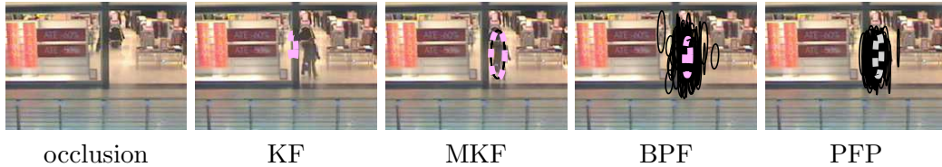
b) In the sequence "ShopAssistant1front" the person gets occluded by walking behind the pillar, frame 80 shown left (zoom in). The tracking results after the occlusion at frame 175 are shown right. KF fails.
