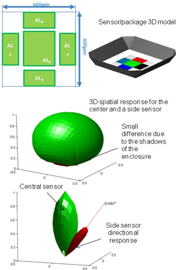
Fig. 2. Integrated light sensors lay out (top), 3D model including enclosure and spatial response of different sensors.
