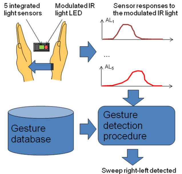
Fig. 1. Interactive air-gesture system using modulated IR light.
