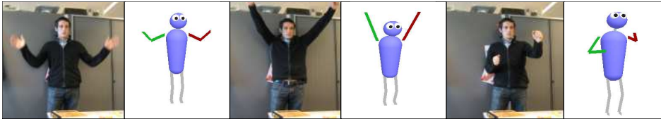
Fig. 5. Example body poses as seen by one of the camera and the avatar showing the resulting 3D reconstruction computed in real-time. For presentation purpose we draw shoulders at fixed distance from the head and elbows in the head-shoulder-hand 3D plane with a proper upper-lower arm length.
